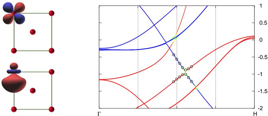
Figure 1: Left: WFs for bcc Fe. Right: Wannier-interpolated bands of bcc Fe along  $\Gamma$ -H. The bands are color-coded according to the value of  $\langle S_z \rangle$ : red for spin up and blue for spin down. The energies are given in eV and the Fermi level is at 0 eV. The vertical dashed lines indicate  $k$ -points on the *ab-initio* mesh used for constructing the WFs. For comparison, points from a full *ab-initio* calculation are shown as open circles.
